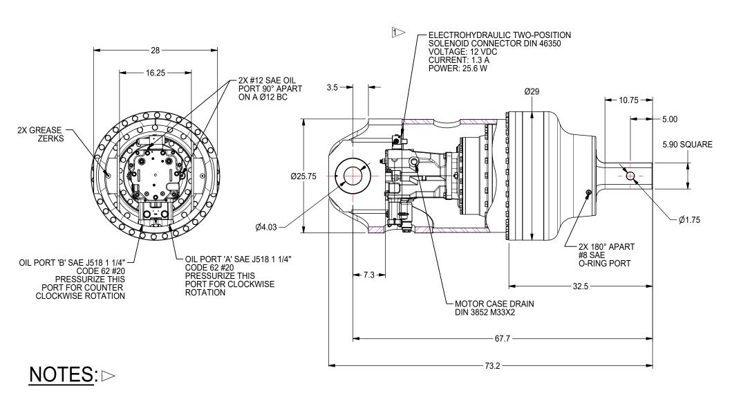
1. MOTOR DEFAULTS TO MAXIMUM DISPLACEMENT. ACTIVATE SOLENOID FOR MINIMUM DISPLACEMENT.
