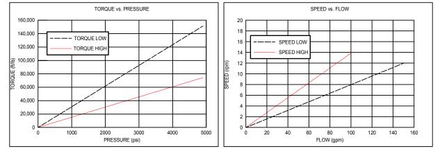
TORQUE AND SPEED CHARTS ARE BASED ON ANALYTICAL CALCULATIONS THAT USE AVERAGE GEARBOX AND MOTOR EFFICIENCIES. STARTING TORQUES ARE APPROXIMATELY 25% LESS THAN RUNNING TORQUE. SYSTEM BACK PRESSURE WILL REDUCE THE RUNNING TORQUES PROPORTIONALLY.
