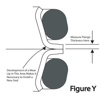
The measured parameter used to check the remaining seal life is flange thickness, at the outer edge (once any wear lip is removed). The measurement must be made carefully because the shoulder is only 0.06" (1.52 mm) from the edge of the flange.
