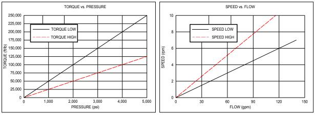
TORQUE AND SPEED CHARTS ARE BASED ON ANALYTICAL CALCULATIONS THAT USE AVERAGE GEARBOX AND MOTOR EFFICIENCIES. STARTING TORQUES ARE APPROXIMATELY 25% LESS THAN RUNNING TORQUE. SYSTEM BACK PRESSURE WILL REDUCE THE RUNNING TORQUES PROPORTIONALLY.
