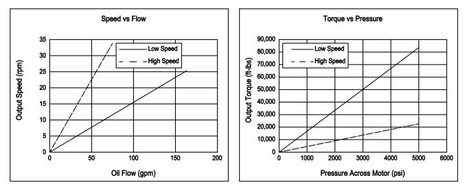
TORQUE AND SPEED CHARTS ARE BASED ON ANALYTICAL CALCULATIONS USING GEARBOX AND MOTOR EFFICIENCIES. SPEED VS. FLOW CHART SPECIFIES MAX-IMUM FLOW AND SPEED VALUES FOR THE DRIVE. STARTING TORQUES ARE APPROXIMATELY 25% LESS THAN RUNNING TORQUE. SYSTEM BACK PRESSURE WILL REDUCE THE RUNNING TORQUES PROPORTIONALLY.
