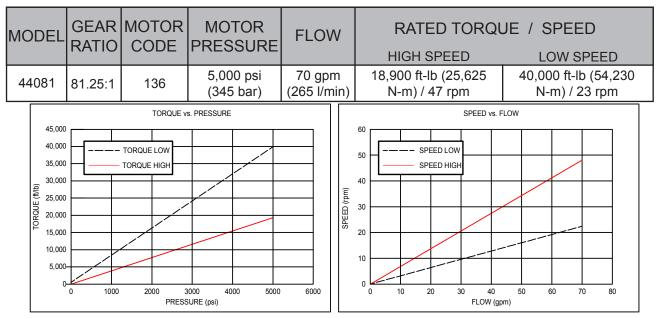
TORQUE AND SPEED CHARTS ARE BASED ON ANALYTICAL CALCULATIONS THAT USE AVERAGE GEARBOX AND MOTOR EFFICIENCIES. STARTING TORQUES ARE APPROXIMATELY 25% LESS THAN RUNNING TORQUE. SYSTEM BACK PRESSURE WILL REDUCE THE RUNNING TORQUES PROPORTIONALLY.
