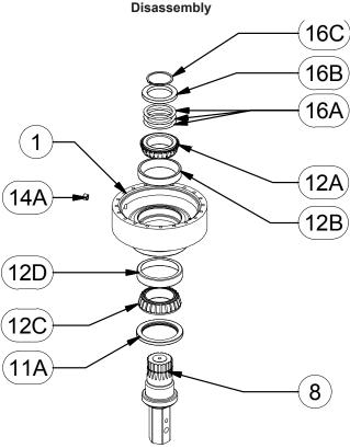
1) Remove the retaining ring (16C), support ring (16B) and shims (16A).
