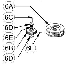
Rotate planet gears (6B) to check for abnormal noise or roughness in bearings (6E) or planet shafts (6C). If further inspection or replacement is required, proceed as follows.
