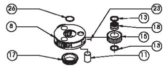
As with the primary planet carrier, check for abnormal noise in the planet gears bearings (18) by rotating the planets and listen and feel for any noise or roughness. If further inspection or replacement is required, follow the same procedure as steps 1-6 of the primary planet carrier assembly. Substitute items as indicated: planet gears (15), planet bearings (18), planet shafts (11), washers (13), carrier (8).
