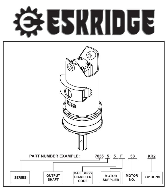
Series 78 Planetary Automatic Kickdown Auger Drive Service & Repair Manual
