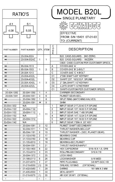
NOTE \* BEARING PRELOAD DETERMINES QUANTITY OF SHIMS. SEAL KIT; P/N 20-016-0501; INCLUDES ITEMS 29 AND 30.
