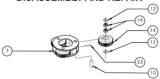
Rotate planet gears (14) to check for abnormal noise or roughness in bearings (19) or planet shafts (10). If further inspection or replacement is required, proceed as follows.
